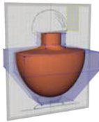
Scan and import sketch, and quickly make a model using SubD surfaces
