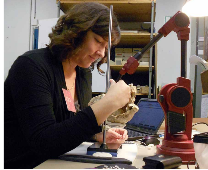
Terhune taking 3D landmarks from a skull using the MicroScribe at the State Museum of Natural History in Stuttgart, Germany.
